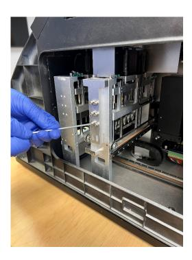
Step 7: Align and prepare to pleace the door panel back on. Align the hinges into the slots and slide the door back into place to the left.
