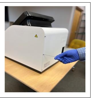
Step 2: Lift the door up slightly, pushing the side door to the right.
