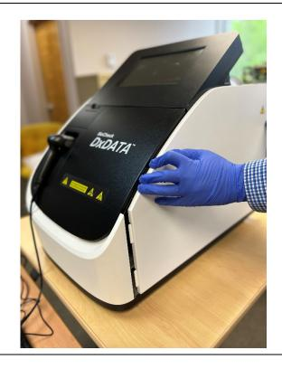
Step 3: Lift the door away from the instrument until you see the hinge below
