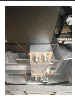
Step 5: Slide the interior mechanism forward towards the front of the instrument.
