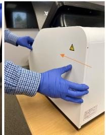
Step 7: Make sure the door is properly aligned on the front seam of the instrument.
