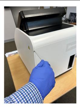
Step 9: Make the back plate is aligned and screwed tightly.
